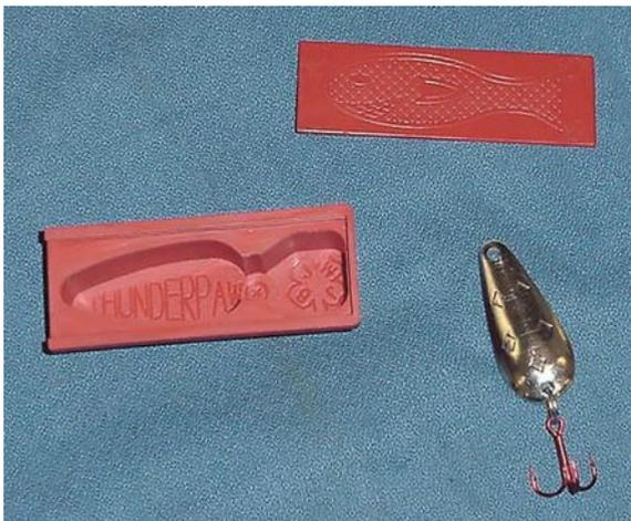
**Students made an injection mold to create the plastic case for the fishing lure. Programmed by a CVTC student in Mastercam and produced on a Haas CNC mill.**
