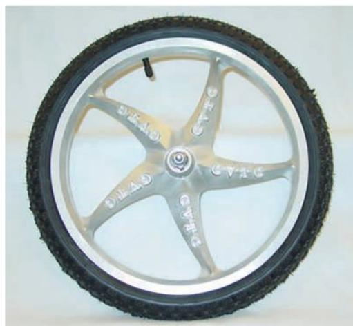
**Above, aluminum bike wheel programmed by a CVTC student in Mastercam and produced on a Haas CNC mill.**
