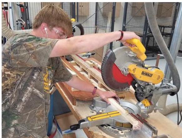
A student demonstrates the correct and safe operation of a miter saw.
