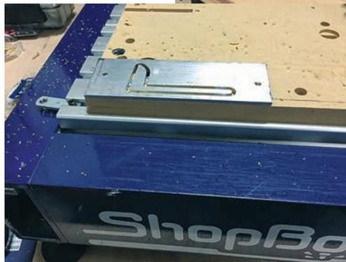
Aluminum cam lever being cut on a ShopBot Desktop
