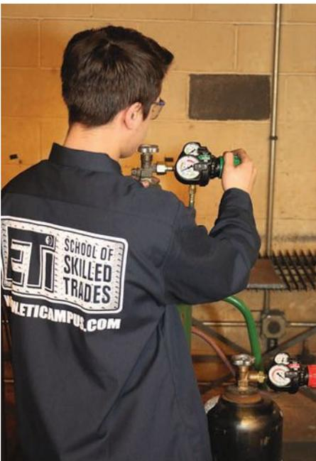
When setting gas flow rates, consult the manufacturer's tip chart. For the Victor 1-101 Series size #1 tip is used here, set oxygen flow at 30 to 35 CFH and acetylene flow at 3 to 5 CFH
