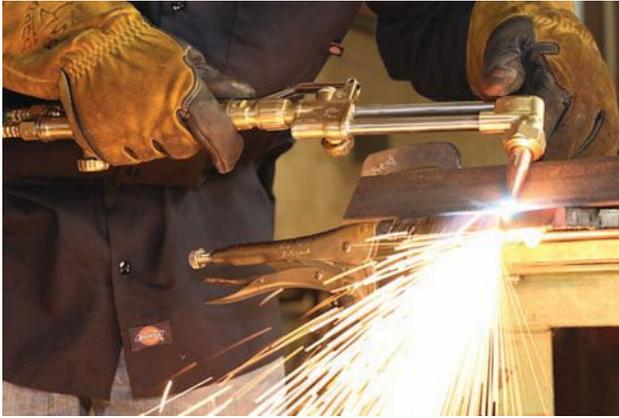
The major equipment manufacturers design equipment so that it is inherently safe to use. For example, this premium torch features built-in check valves and flashback arrestors.
