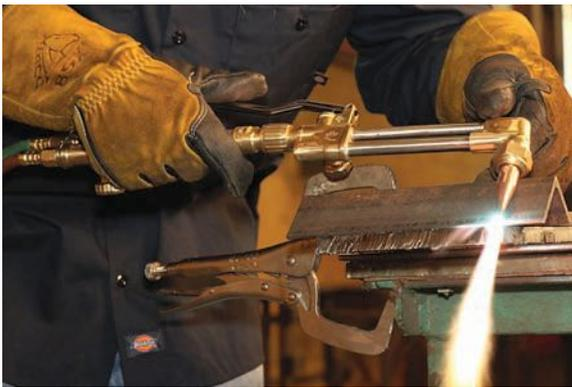
Hold the torch about 1/8 in. off the plate and at the edge of the plate until the steel reaches its kindling temperature, as indicated by a cherry red color.
