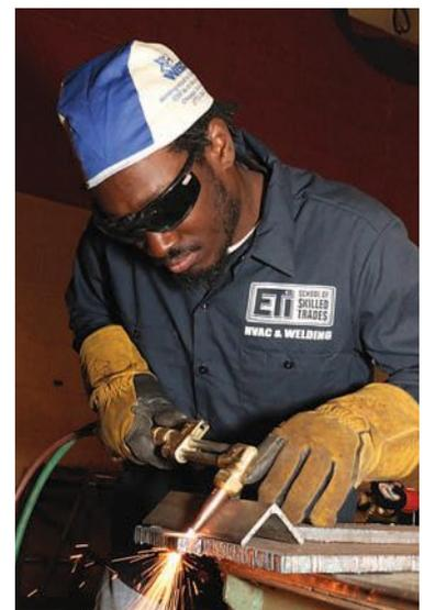
To bevel an edge, the operator uses a piece of angle iron and keeps it in place with another plate.
