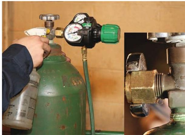
After setting flow rates, spray connections with soapy water. If a soap bubble occurs (see inset), tighten the connection and re-adjust flow rates if necessary.
