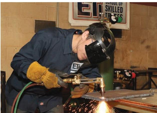
Use your offhand to brace the torch. You can push or pull the torch depending on the situation, but in any event, tilt the head of the torch about 5° in the direction of travel.
