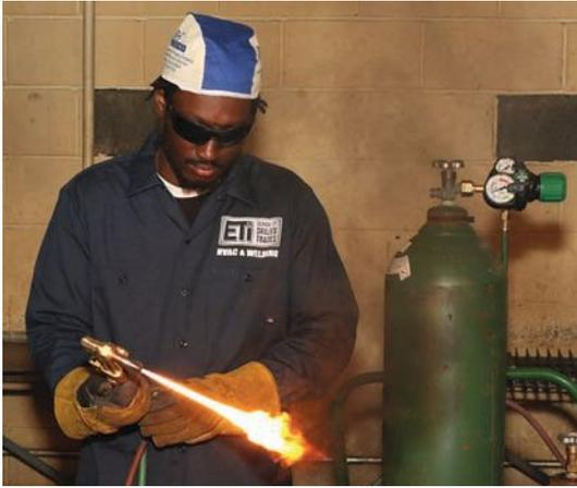
After lighting, the flame will generate a lot of soot and smoke. Continue opening the fuel valve until the smoke disappears.
