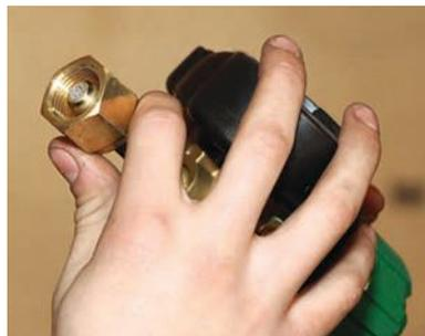
Visually inspect all threaded connections for signs of damage and contamination by grease, oil, or particles. Under high pressure and in the presence of oxygen, contaminants can easily combust.
