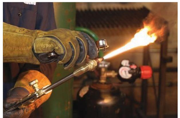
Open the oxygen valve on the torch handle all the way to ensure maximum flow to the cutting valve, open the acetylene valve 1/4-turn, and ignite the torch with a spark lighter, holding the lighter off to the side of the tip.
