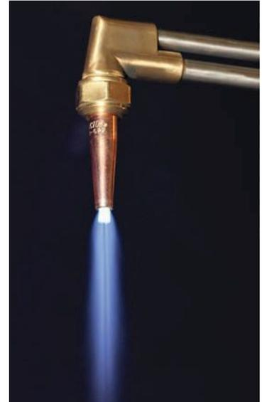
After the soot disappears, transfer to the oxygen valve on the cutting attachment and slowly add oxygen until establishing a bright neutral pre-heat flame. Depress the oxygen cutting lever and release it; if necessary, re-adjust the oxygen level so that the flame shows both good pre-heat cones and a good cutting oxygen stream.
