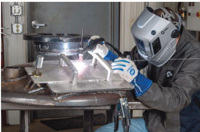
**Proper heat input is a critical factor in successfully welding aluminum with GTAW. Aluminum is conductive, so the heat of the weld puddle can be pulled away quickly. This requires putting in a lot of heat to establish the weld puddle, but controlling that heat is key to preventing a runaway puddle or burn-through.**
