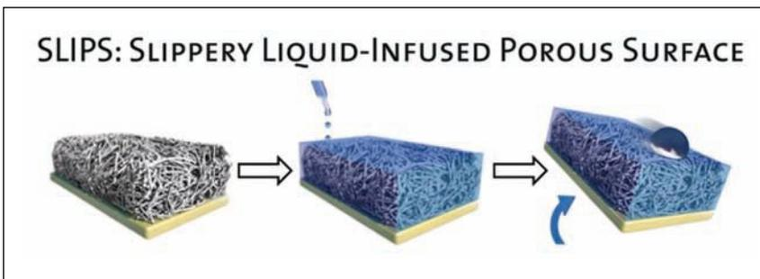
**Fig. 1**—The figures show openings that would be invisible unless you were looking at the object under an electron microscope. To infuse SLIPS, the outer layer of a metal or ceramic material would need to have micro-sized openings that serve as SLIPS wells to self-heal the outer coating if it is damaged.
