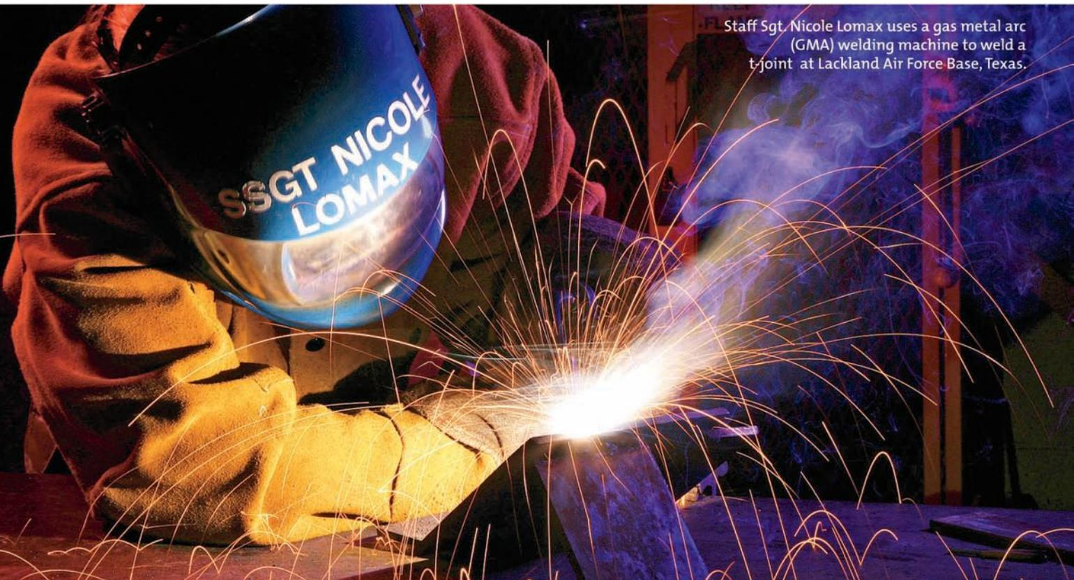
Staff Sgt. Nicole Lomax uses a gas metal arc (GMA) welding machine to weld a t-joint at Lackland Air Force Base, Texas.
