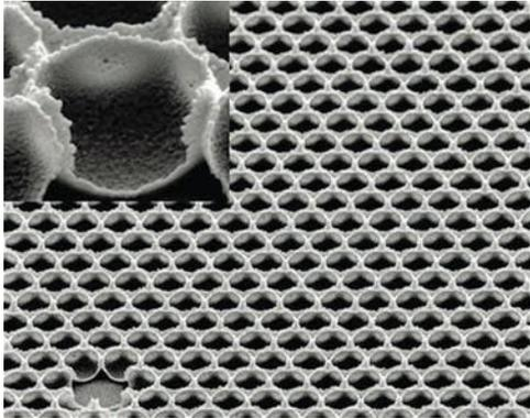
**Photo 4**—To create the self-cleaning superglass, the Wyss Institute scientists needed to create a sheet of glass with a middle layer that contained a honeycomb of micro-sized wells into which they infused SLIPS. To see these opening you would need to view the glass under an electron microscope.
