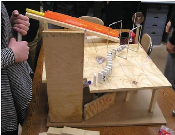
**Photo 4—Part of one Rube Goldberg machine showing dominoes and a Newton's Cradle**
