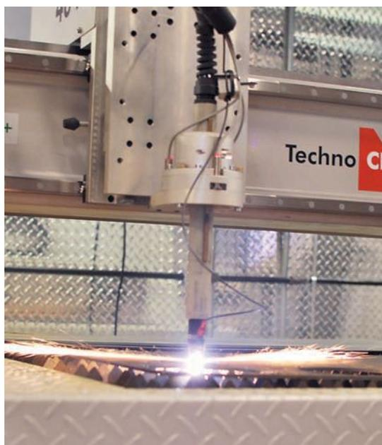
**Metal cutting project in the works on the classroom's Techno CNC plasma cutter**
