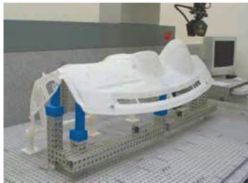
**Hyundai Mobis 3D printed an instrument panel in ABS plastic to measure component fit.**
