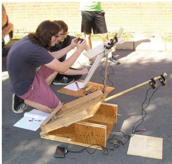
**Photo 1—Ben Rudnik and Nathan Schweitzer test and video record their golf ball launching machine. Another machine in the foreground clearly shows the photogates and LabQuest unit.**
