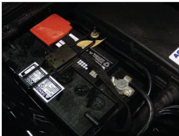
manufacturer that is producing cars today. Of course, that list would be even longer. The point of the list is to show that it is quite possible that just disconnecting a battery will require some sort of calibration or code clearing.
