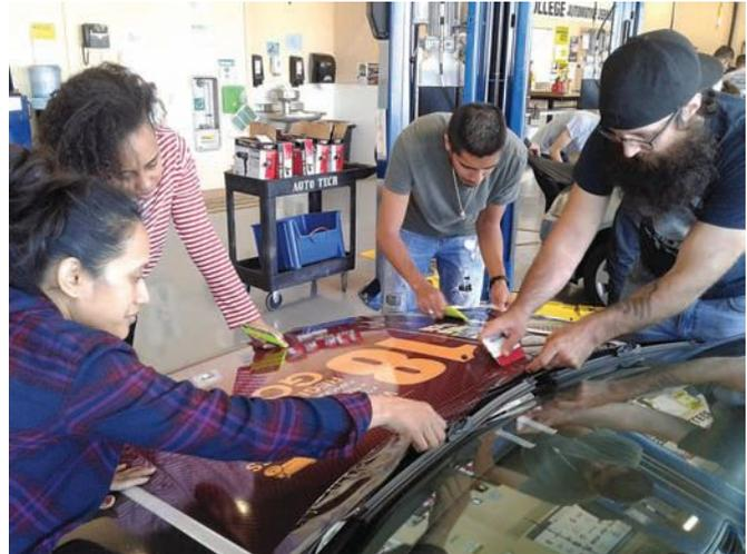
Below, students use specially designed squeegee tools to smoothly install the adhesive graphic film.
