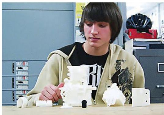
Silverman reverse engineered Briggs & Stratton small engine parts and printed physical models on Chico Unified’s Dimension 3D Printer.
