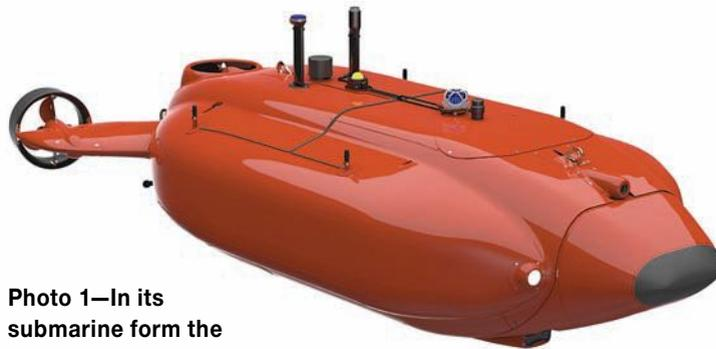
**Photo 1—In its submarine form the Aquanaut Transformer has an aerodynamic shape which allows it to easily move through water.**
