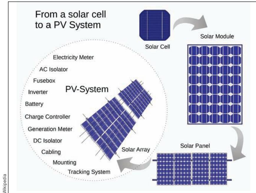
Fig. 2—PV cells are combined into modules then into panels to form end products.
