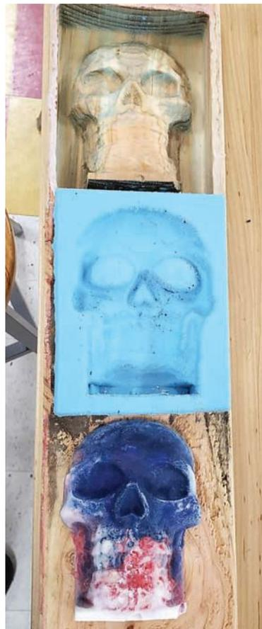
puter. Many of the same files that can be used with a 3D printer can be 3D carved on a ShopBot, and the resulting model can be used to create molds to aid in the production of many copies.
