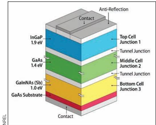
**Fig. 4—Multi-junction TFPV cell internal structure**
