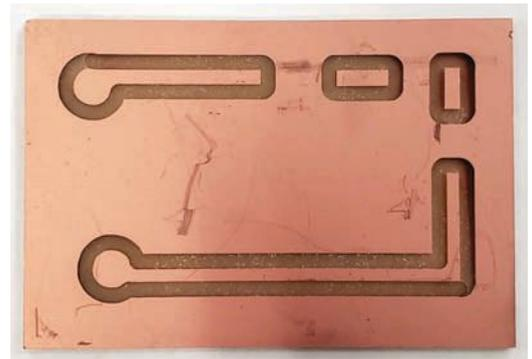
PCB blank with a thin layer of copper on the board, machined on the ShopBot PRTalpha with a 1/16" bit
