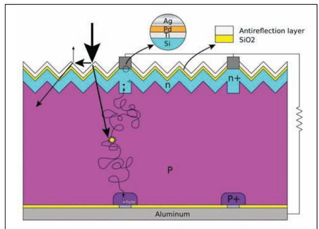
**Fig. 1—Single-junction PV cell operation: Photons of appropriate energy liberate electrons, which cross the semiconductor junction and generate a potential difference.**
