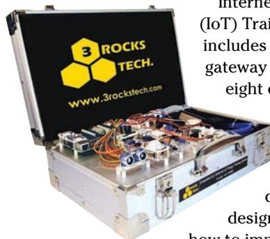
Internet of Things (IoT) Trainer, IoT-16900 includes a CPU board, gateway (Raspberry Pi), eight different sensors, and seven actuators. It is a training system for students to learn IoT design principles and how to implement IoT applications. A farm management application is included for users to be familiar with the system.
