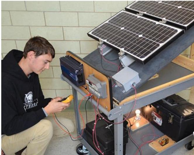
**Using energy converted using a portable photovoltaic system, a Bridging Communities student determines the load on the circuit powered by the 12 V battery.**
